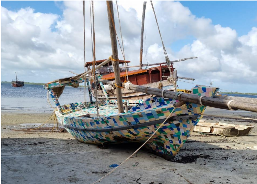
Plate 14: Boat made from recycled plastics by the Takataka Heroes
