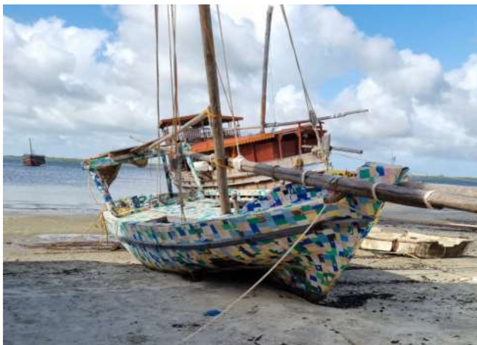
Plate 14: Boat made from recycled plastics by the Flip-flopi
